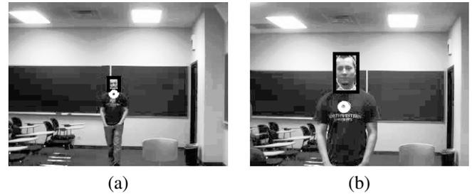
Fig. 11. a) System locked on to chest when subject is initially far away, and b) System locked on to chest when subject is moving closer.
