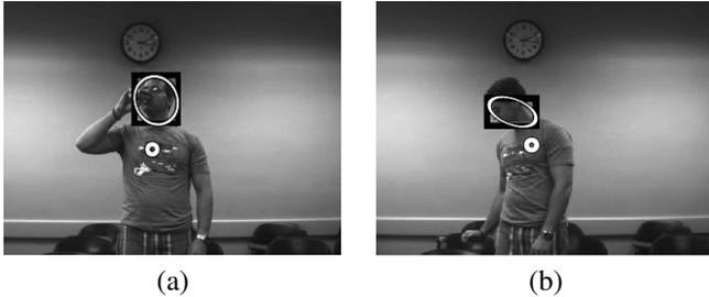
Fig. 13. a) System handling occlusion of area that is being tracked, and b) System handling a pose change while maintaining proper aim at the subject's chest.
