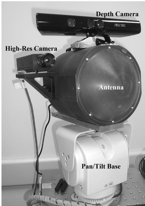
Fig. 1. Setup of system, including the antenna, the high-resolution camera, the depth camera, and the pan/tilt base.
