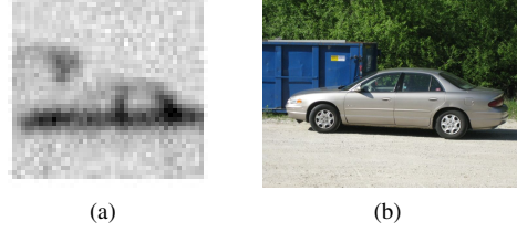
Fig. 3. (a) PMMW test image, and (b) visible light image of the same scene.
